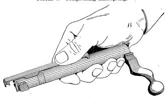
FIGURE 8.—Removing extractor.
